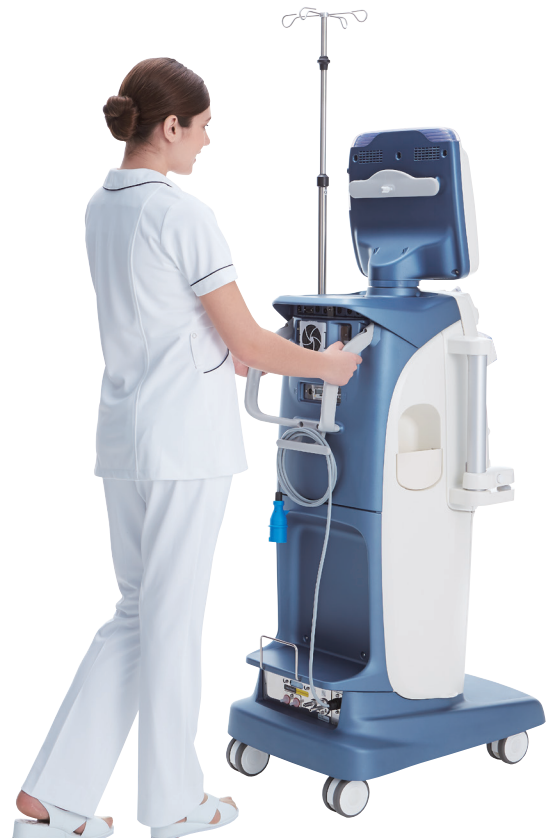
A well laid-out extracorporeal circuit minimises patient extracorporeal blood volume and makes it easy to install the bloodline set.
