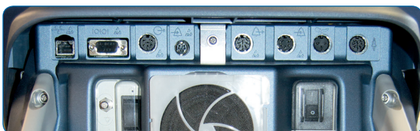
Interface hub for connecting network and various alarm in- and outputs. Also available is the unique Publicly Available Specification connection port for external alarming device (IEC PAS 63023).
