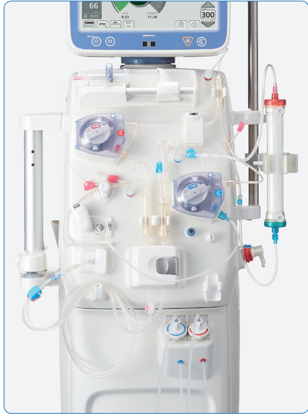
A well laid-out extracorporeal circuit minimises patient extracorporeal blood volume and makes it easy to install the bloodline set.
